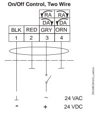
Figure 10: Control Wiring Diagrams
