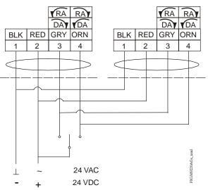
Floating Control, Four Wire with Tandem Connection
