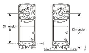
Figure 5: Positioning the Anti-Rotation Bracket (See Table 2.)
