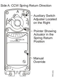
Figure 2: Side A of Actuator
